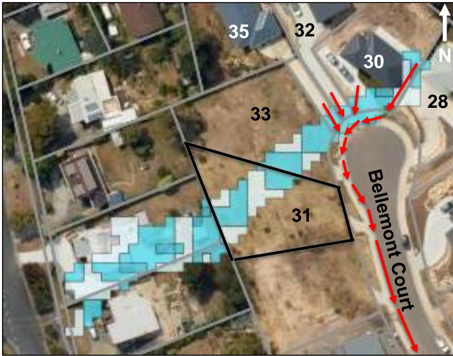
Figure 5: Council flood model extent at 31 Belmont Court, Geilston Bay [3], red arrows indicate direction of water flow post-subdivision
