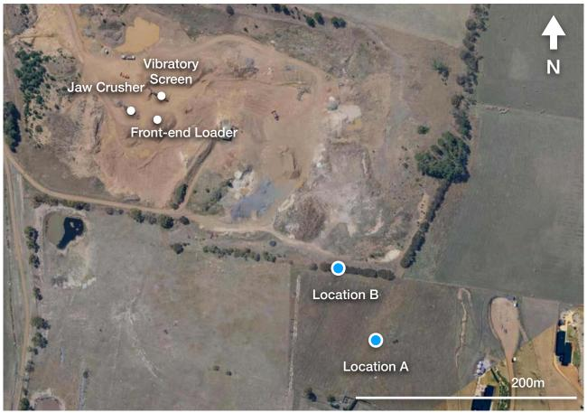
FIGURE 2.1: MODELLED NOISE SOURCES AND MEASUREMENT LOCATIONS
