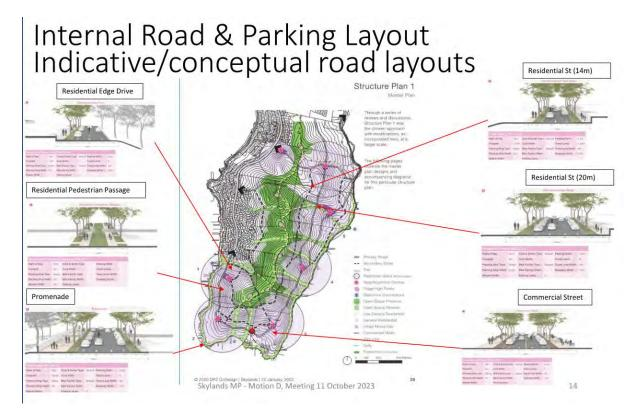
Figure D - Location and typical cross sections of the different roads within the Skylands MP, showing on-street car parking options.
