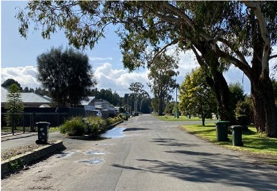
Plate 2. Looking northeast along Woodhurst Road past Leyden Avenue (right middleground) on 20 August 2022 after most of the flood waters had evaporated, and slowly infiltrated the subsoil via stormwater gratings. Compare with Plate 1. The water level in the gratings was at ground level, indicating the water table in the immediate vicinity of the line of gratings is at surface, but it may not be at surface further from the road.
