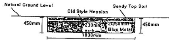
MODIFIED ABSORPTION TRENCH DETAIL Fig 2
